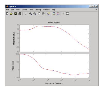
As the overlap of the curves in the figure shows, the reduced model provides a good approximation of the original system.
