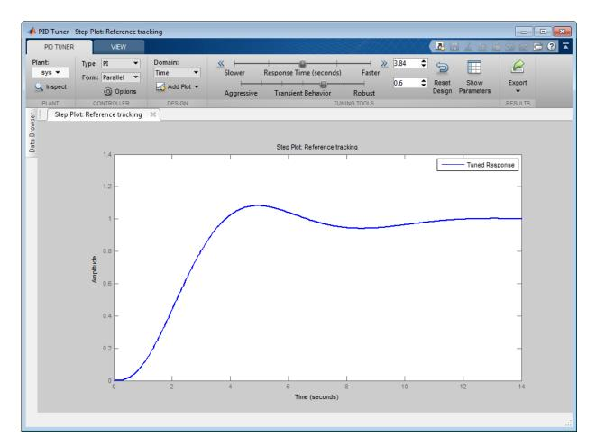
When you open **PID Tuner**, it automatically designs a controller of the type you specify (here, PI). The controller is designed for a balance between performance (response time) and robustness (stability margins). **PID Tuner** displays the closed-loop step response of the system with the designed controller.
