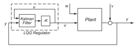
The plant in this model experiences disturbances (process noise) w and is driven by controls u. The regulator relies on the noisy measurements y to generate these controls. The plant state and measurement equations take the form of
