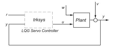
The plant has three states (x), two control inputs (u), two random inputs (w), one output (y), measurement noise for the output (v), and the following state and measurement equations:
