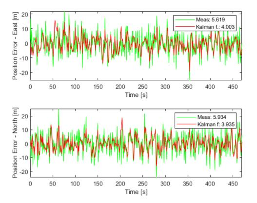
The plot legends show the position measurement and estimation error  $(||x_e - \hat{x}_e||_1)$  and  $||x_n - \hat{x}_n||_1$  normalized by the number of data points. The Kalman filter estimates have about 25% percent less error than the raw measurements.
