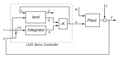
The servo controller you design ensures that the output y tracks the reference command r while rejecting process disturbances w and measurement noise v.
